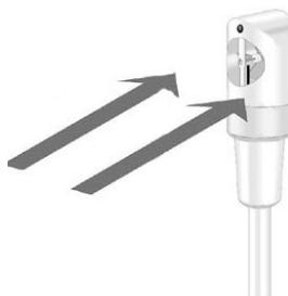
The correct measuring value is determined by rotating the probe slightly in both directions until the maximum value is displayed.
