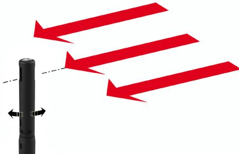
The correct measuring value is determined by rotating the probe slightly in both directions until the maximum value is displayed.
