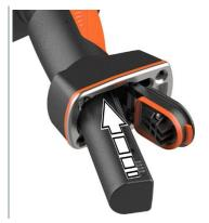
5 Close the battery compartment cover and secure with the unlocking button.
