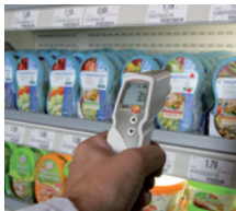
Infrared measurement refrigerated shelving
